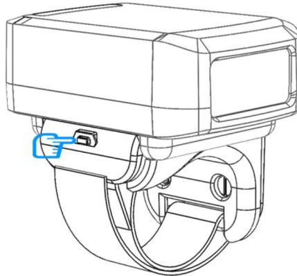
**Figure 2** Push Trigger Assembly Latch In
