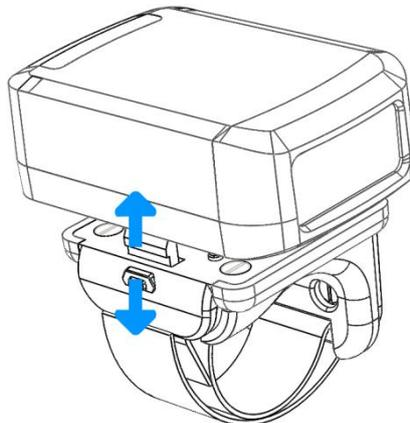
**Figure 3** Lift Trigger Assembly Off LR50
