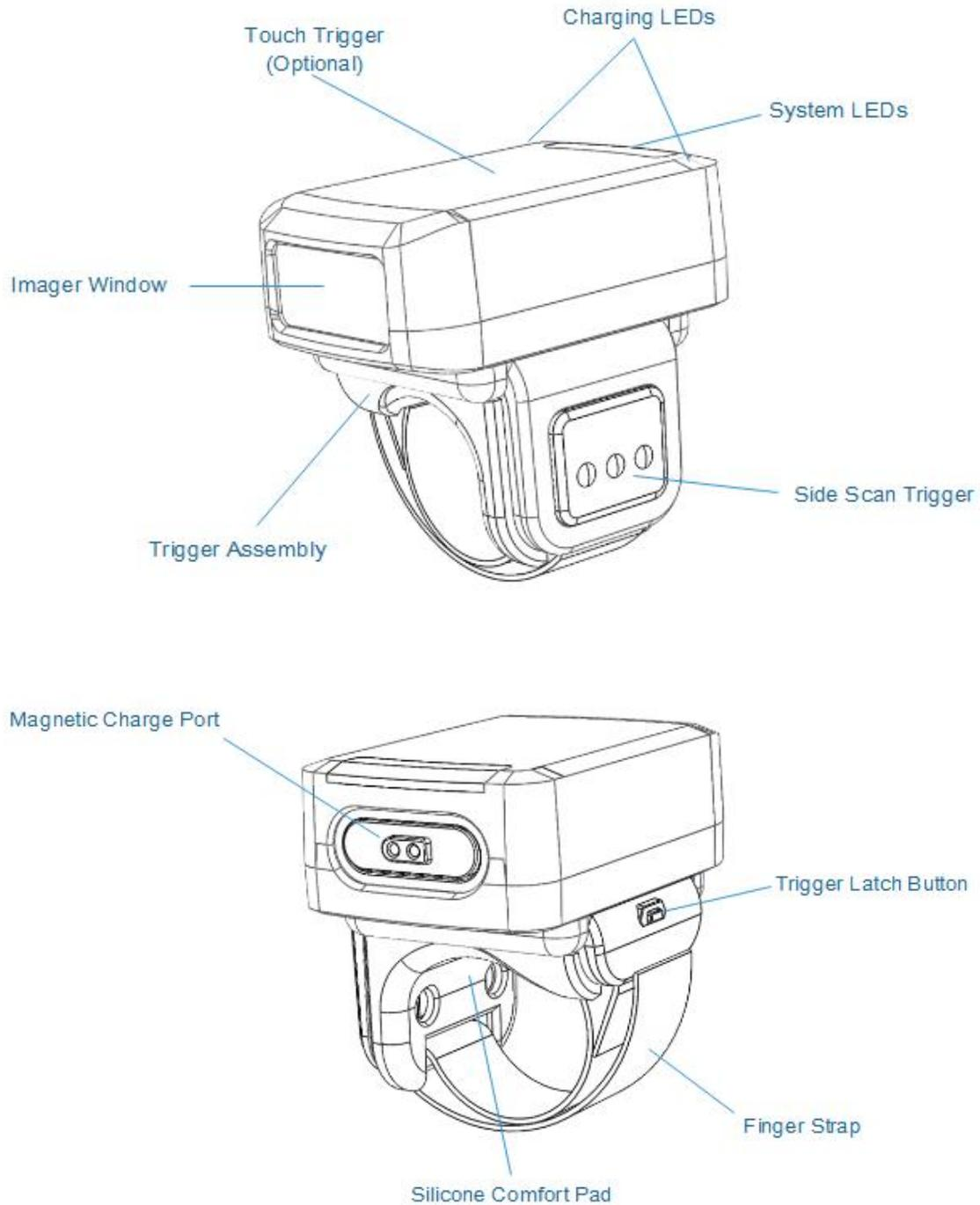
**Figure 1** LR50 Series Configuration Features
